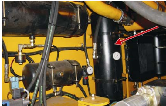
Remove receiver tank
