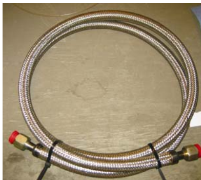
Install SS hose
