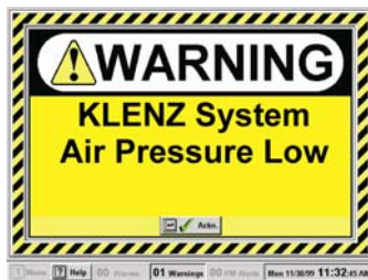
Massive air leak
