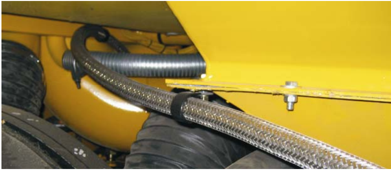
Stainless steel hose mounted to bottom corner of blower housing
